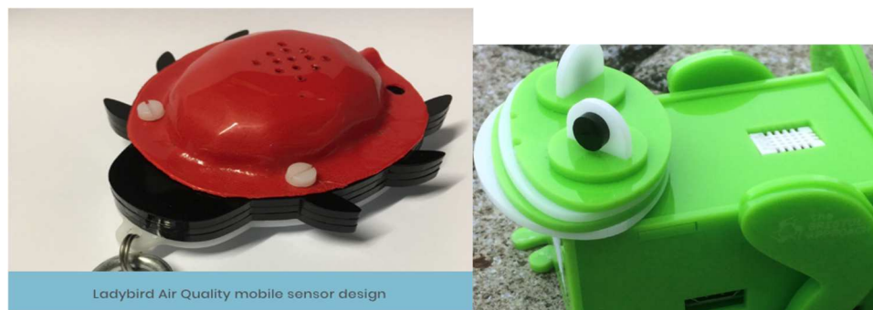
Figure 46 Prototype Ladybird air quality sensor from the air quality pilot; prototype FrogBox temperature and humidity sensor from the damp homes pilot
