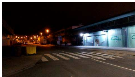
Figure 2 – HPSV Conventional lighting
